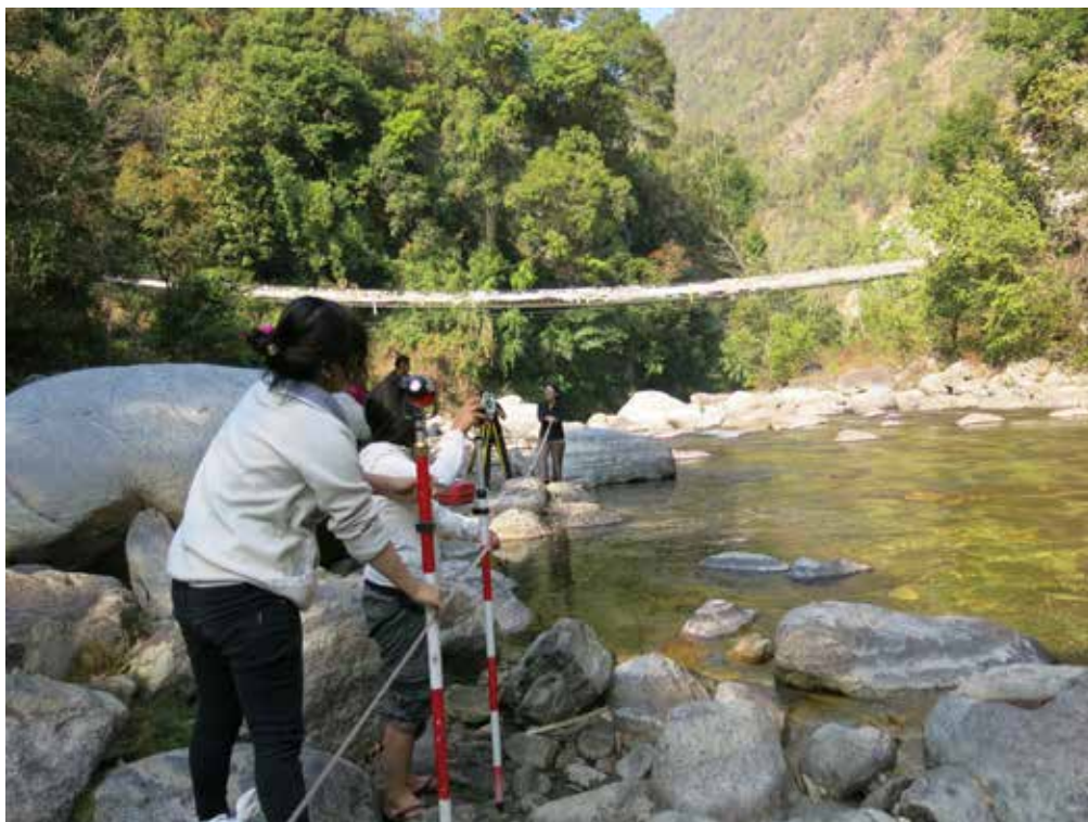
Fig. 16 Measuring Water Level at Nyera Amari HPP
